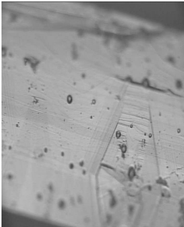
Figure 2 The microstructure on the surface of ZrS_3 single crystal
