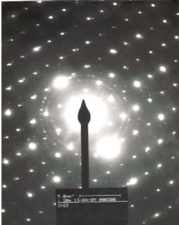
Figure 4 The SAD pattern of as grown ZrS 3 single crystals
